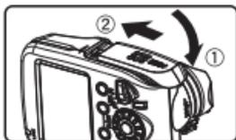
**3. Close the battery:** Close the battery Compartment cover and slide it up.
